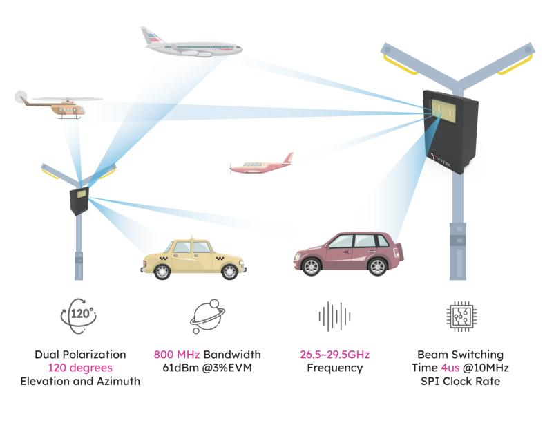
Y. Beam S is a 28GHz 5G mmWave antenna array front-end module dedicatedly developed for the high-speed data conversion subsystem (HS-DCS) interface of NXP LA1224 Bonnyrigg platform. Y. Beam S internally integrates modulators, demodulators, up/down converters, and beam-formers.
